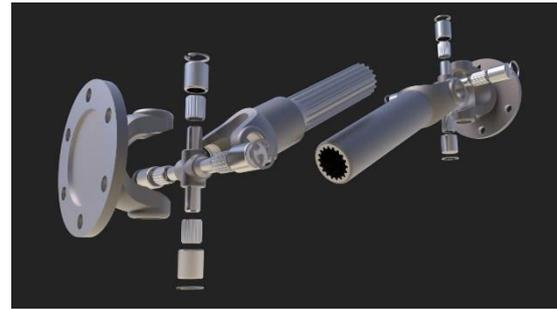
Fig 9. Assembly Of Drive Shaft
